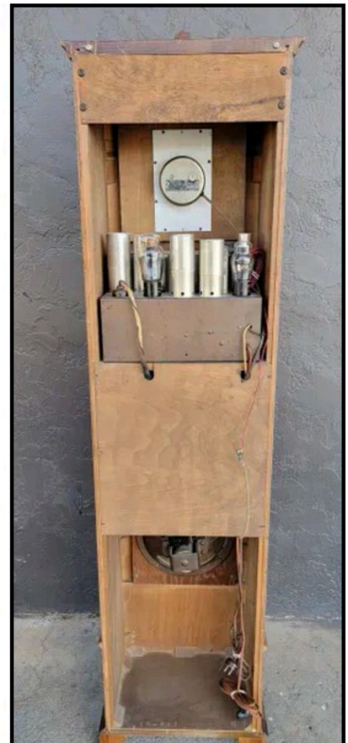
The Back an internal electronics of the 1931 Sears Silvertone Grandfather Clock Radio at the Texas Broadcast Museum
